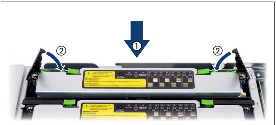
Figure 32: Installing a memory board
